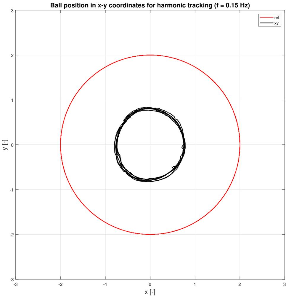
Fig. 6.28 Control results for harmonic tracking in the x-y plane
