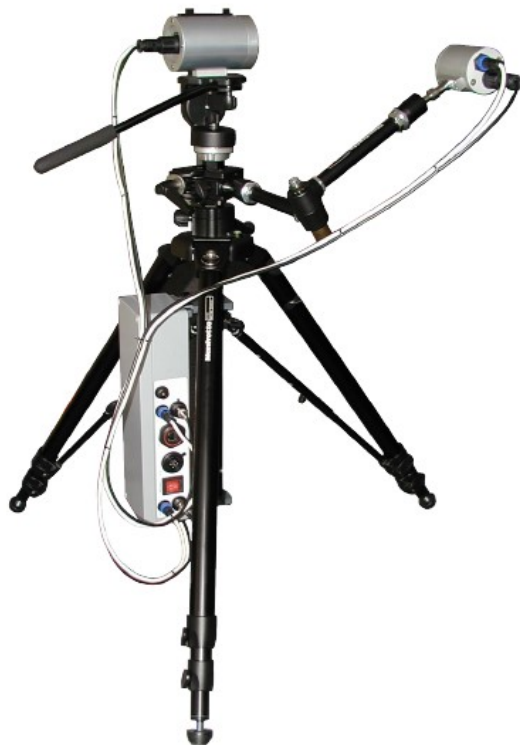
Obr. 5.2.1: Doppler radar system – DRS-1 [45].
