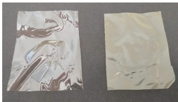
Fig. 14 Appearance of the chitosan films a) without and b) with thyme essential oil/Tween 80
