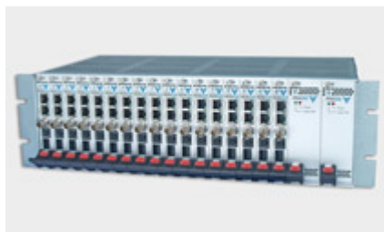
Obr. 13. MPEG-2 koder v rack mounted šasi [39]
